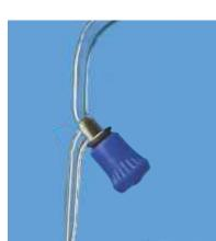
Automatic Zero, Accuracy as per Class A of IS 1997:2008/EN ISO 385, with Reservoir, Rubber Bellow and Boroflo Stopcock, Amber With Certificate
