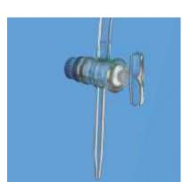
Automatic Zero, Accuracy as per Class A of IS 1997:2008/EN ISO 385, with Reservoir, Rubber Bellow, Glass Stopcock, Amber With Certificate
